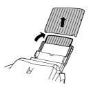
**2** Fan the paper, and then tap the edge against a flat surface to even the stack.
